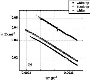
FIG. 1. Transport data collected from the ampullary gel of sharks: (a) I-V traces show Ohmic response at various applied potentials, up to (not shown) 1 V; (b) semilog plot of conductivity vs reciprocal temperature for all three species. Range of temperatures matches range of possible environmental temperatures encountered by elasmobranchs (roughly  $0-30\,^{\circ}$ C).
